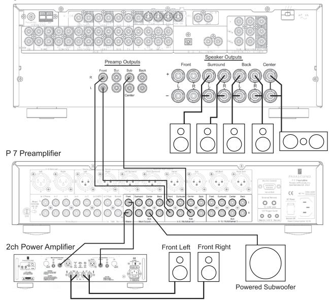
**Note:** When the P 7's Bypass mode is selected, its <u>volume level is fixed</u> and the balance, trims and tone controls are all disabled; these adjustments should be made on the digital surround receiver.
